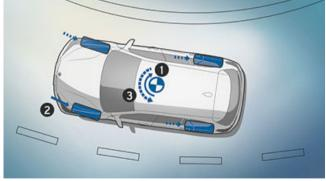
by applying braking pressure asymmetrically when braking
